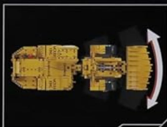
Twist Waist Steering (Electric Control)
