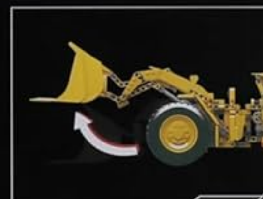
TShovel Arm Can Be Raised and Lowered (Electric Control)
